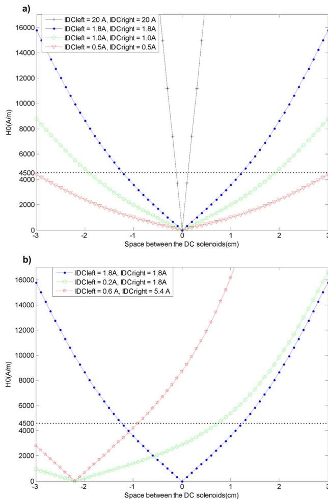
FIG. 4. Simulation of the dc magnetic field strength ( $H_0$ ) between the dc solenoids. 4500 A/m is shown with a dashed line which was the ac magnetic field applied between the dc solenoids. (a) For the solenoid currents of IDCleft=IDCright=0.5, 1, 1.8, and 20 A. (b) For the solenoid currents of IDCleft=1.8 A, IDCright=1.8 A; IDCleft=0.2 A, IDCright=1.8 A; and IDCleft=0.6 A, IDCright=5.4 A.
